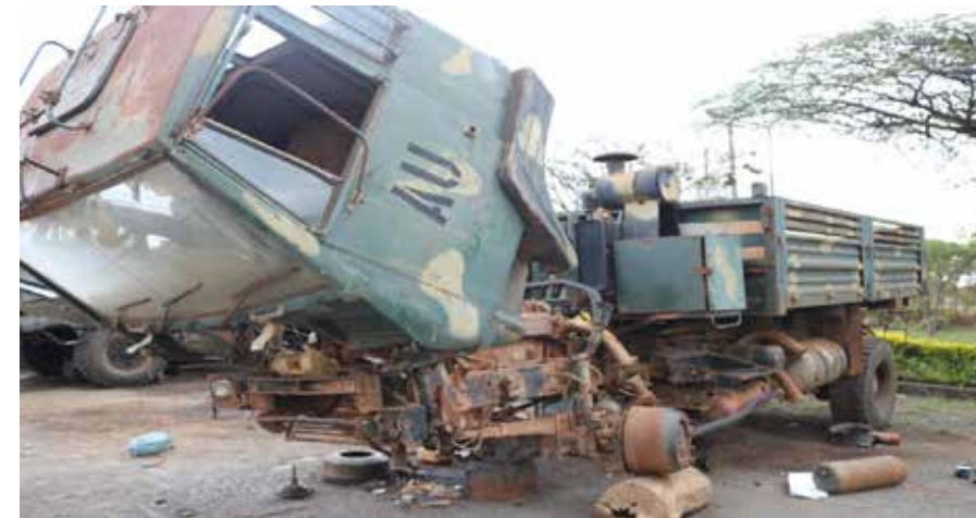
Pic 2: Extensively damaged vehicle awaiting repairs in the field.
